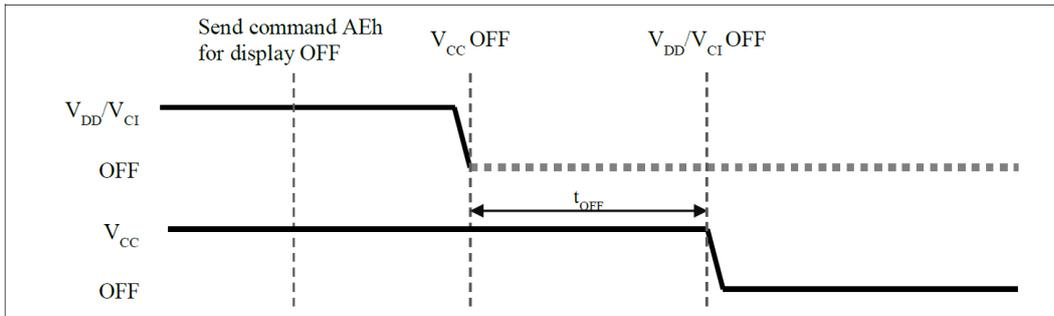
Note:  $V_{CC}$  should be floated when OFF.
