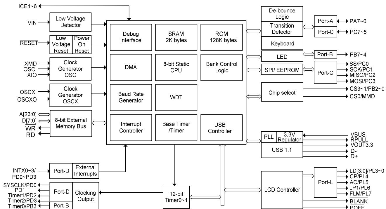
Figure 2-1 ST2203U Block Diagram
