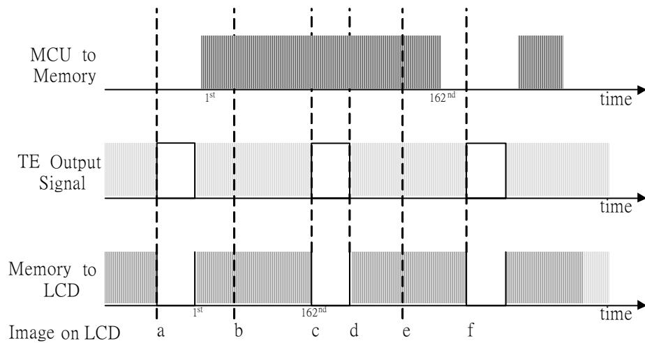
The MPU to Frame Memory write begins just after Panel Read has commenced i.e. after one horizontal sync pulse of the Tearing Effect Output Line. This allows time for the image to download behind the Panel Read pointer and finishing download during the subsequent Frame before the Read Pointer “catches” the MPU to Frame memory write position.
