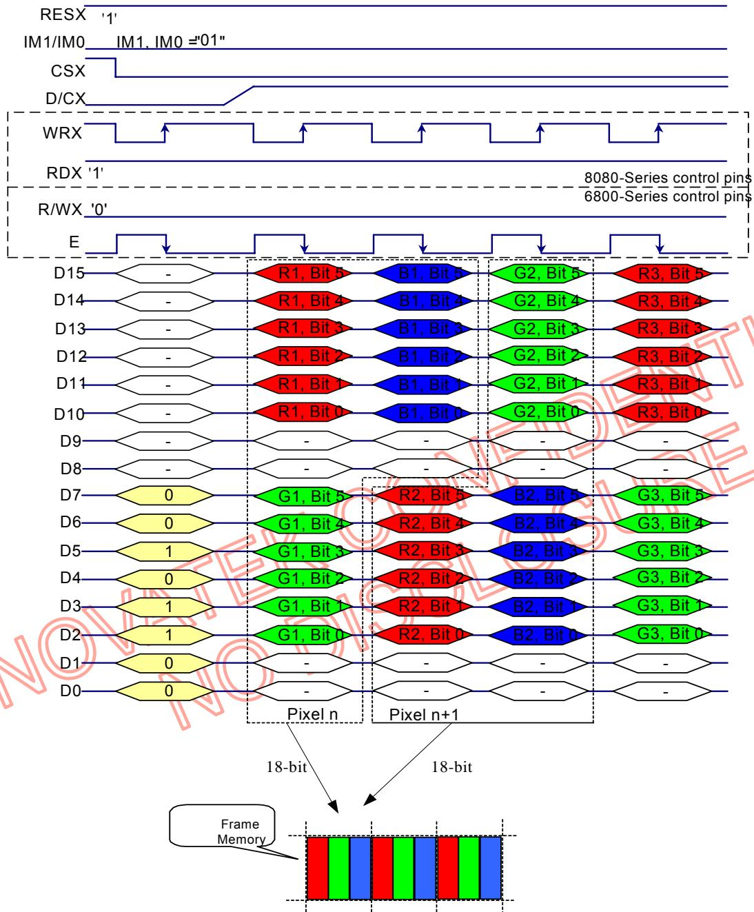
Note 1. The data order is as follows, MSB=D15, LSB=D0 and picture data is MSB=Bit 2, LSB=Bit 0 for Read and Green and MSB=Bit 1, LSB=Bit 0 for Blue data.
