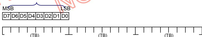
Fig. 8.4.1.1 Serial interface data Stream format
