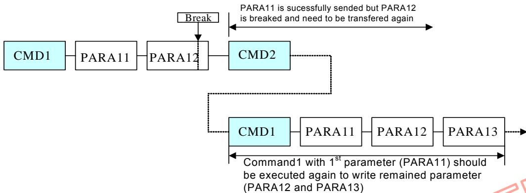
Fig.8.5.3 Write interrupts recovery (serial interface)
