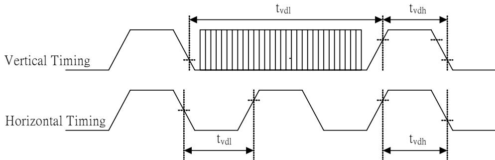
Table 8.3.1 AC characteristics of Tearing Effect Signal
