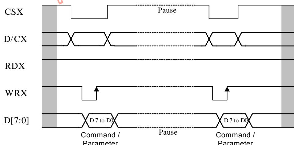
Fig. 8.5.6 Parallel bus Pause Protocol (paused by CSX)
