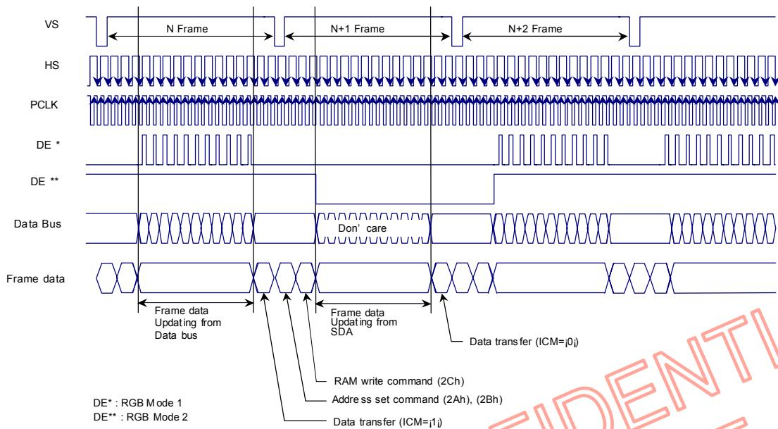
Fig. 7.4.3.2 RAM Access via SPI Interface in RGB Mode (V)
