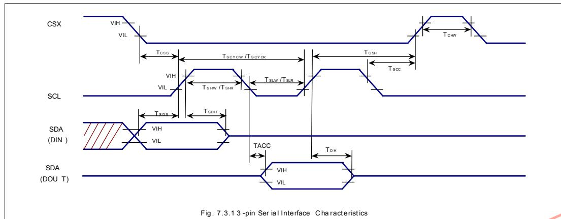
Table 7.3.1: 3-pin Serial Interface Characteristics
