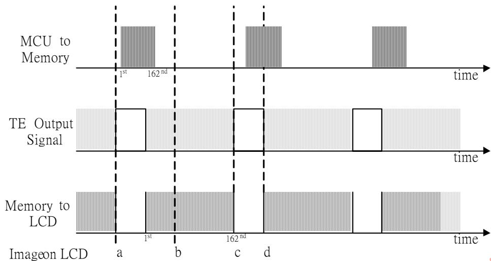
Data write to Frame Memory is now synchronized to the Panel Scan. It should be written during the vertical sync pulse of the Tearing Effect Output Line. This ensures that data is always written ahead of the panel scan and each Panel Frame refresh has a complete new image:
