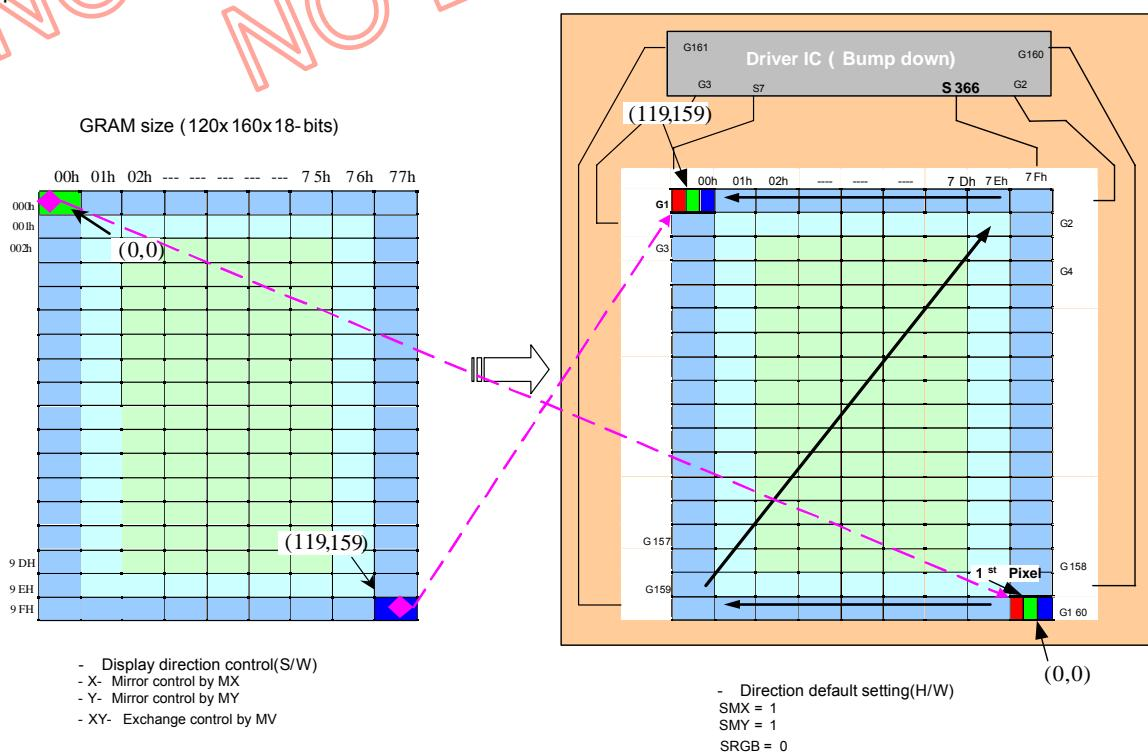
Case 3 of Resolution (128RGB x 128) (GM1, GM0 = "10") RAM size=128 x 128 x 18-bits (Used)
