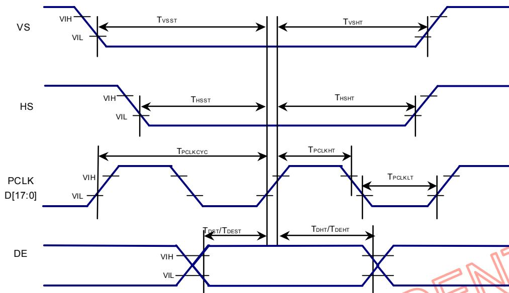
Fig. 7.4.3.1 General Timing for RGB I/F
