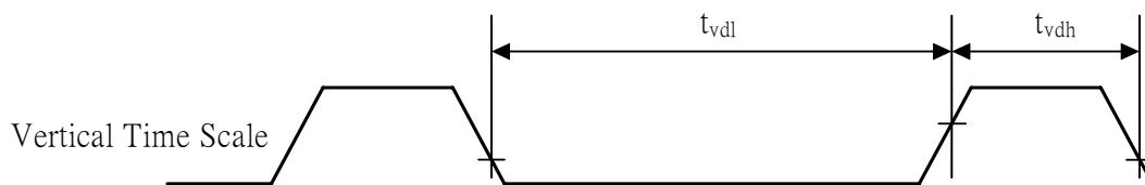
*$t_{vdh}$ = The LCD display is not updated from the Frame Memory*
