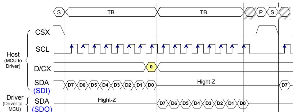
4-pins Serial Protocol (for RDID command: 24-bits read)
