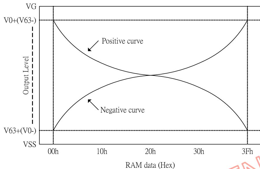
**Fig. 5.9.4 Relationship between RAM data and output level**
