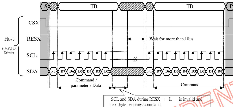
Fig. 8.5.1 Serial bus protocol, write mode – interrupted by RESX
