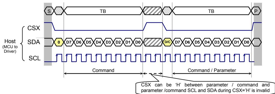
Fig. 8.4.1.2 3-pins Serial interface Write protocol (Write to register with control bit in
