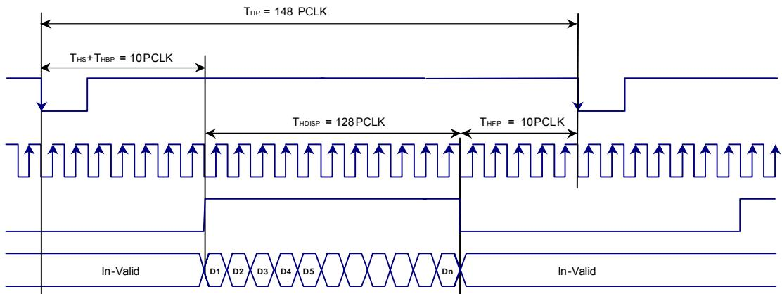
Fig. 7.4.5.3 RGB Mode 2 Horizontal Timing Diagram
