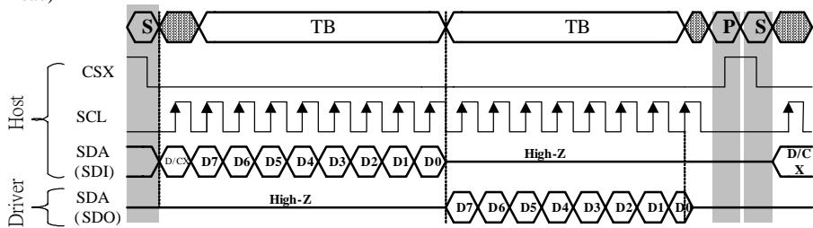
3- Pin Serial Protocol( for RDDID command: 24- bit read)
