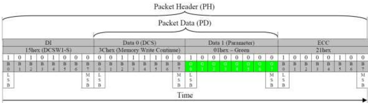
Figure 83: Green Subpixel Write (DCSW1-S) – Example 3
