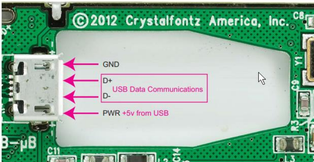
Figure 8. USB Connection Detail
