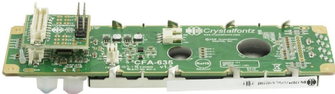
Figure 12. Angled View of CFA-RS232 Level Translator Mounted on CFA735-xxx-KR
