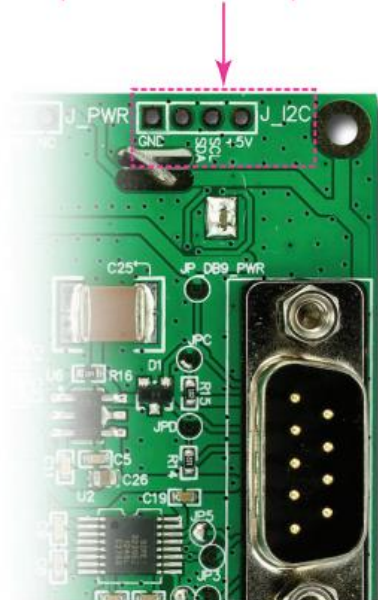
J_I 2 C Expansion Port For 4-pin I 2 C connector
