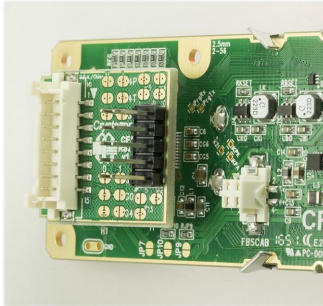
Figure 5. Angled View of CFA-RS232 Level Translator Mounted on CFA635-xxx-KL
