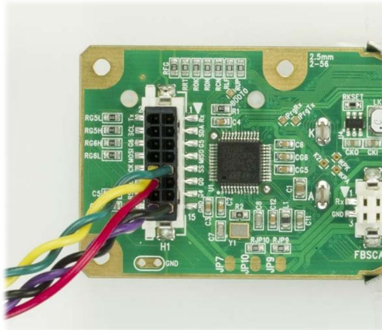
Figure 8. ATX Connection with WR-PWR-Y25 or WR-PWR-Y38 Cable
