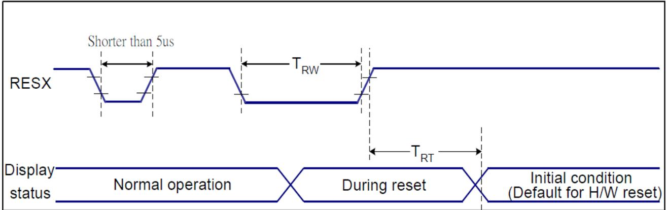
Figure 7 Reset Timing
