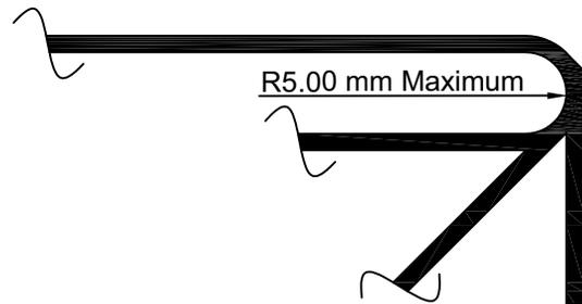
Figure 1. Example Of Minimum Plastic Bend Radius For FPC/FFC
