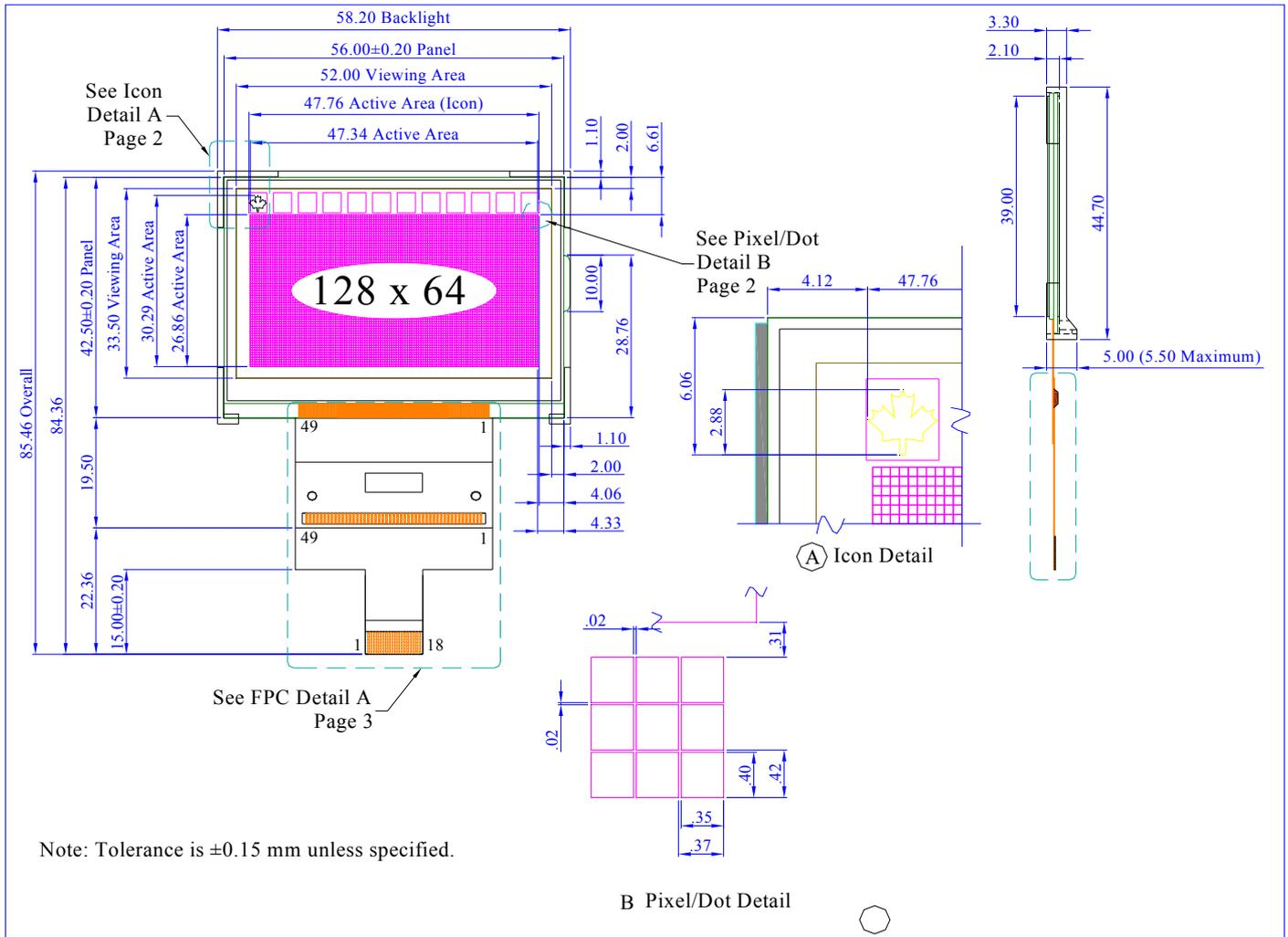
Note: Tolerance is ±0.15 mm unless specified.
