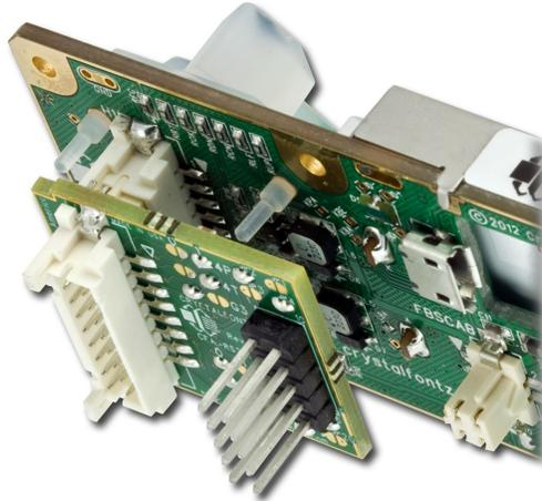
Figure 1. Photo Of CFA-RS232 Mounted On A Compatible LCD Intelligent Module (CFA735)
