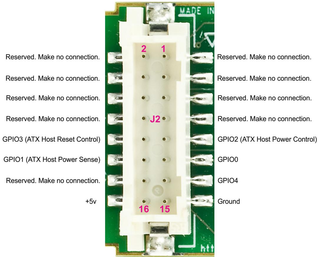
Figure 4. CFA-RS232 “J2” Connector Pin Assignments
