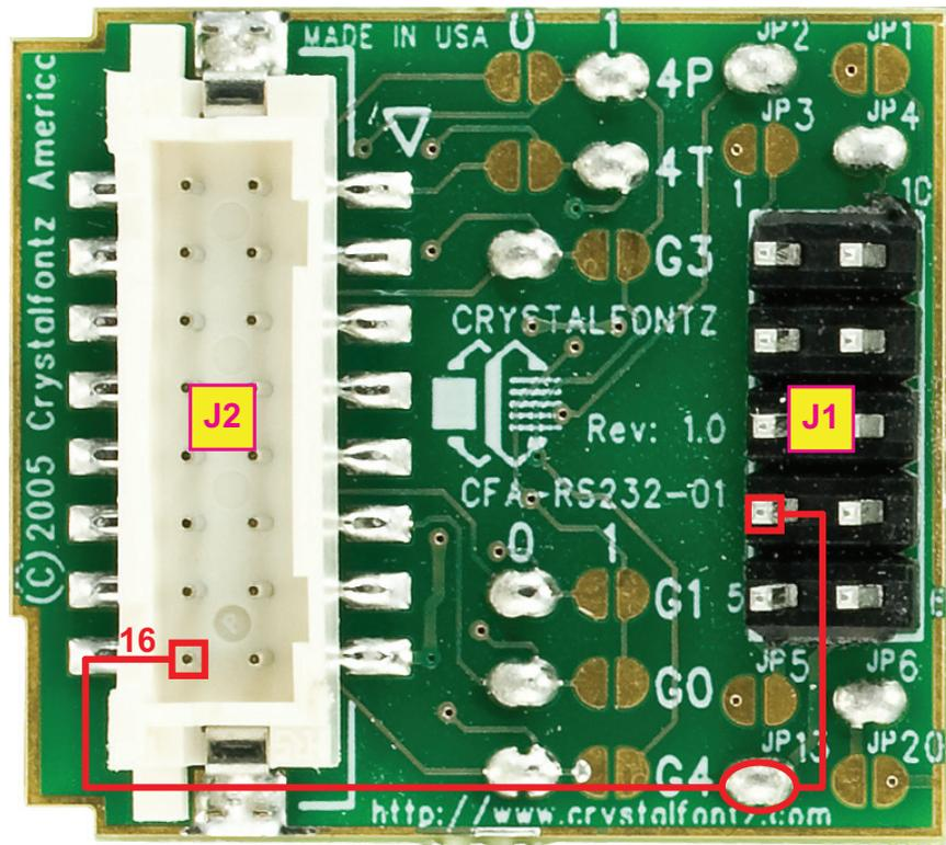
Jumper JP13 is closed by default at the factory. It allows power to be supplied to J1.
