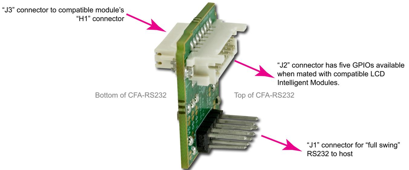
Figure 3. CFA-RS232 Side View of Connectors
