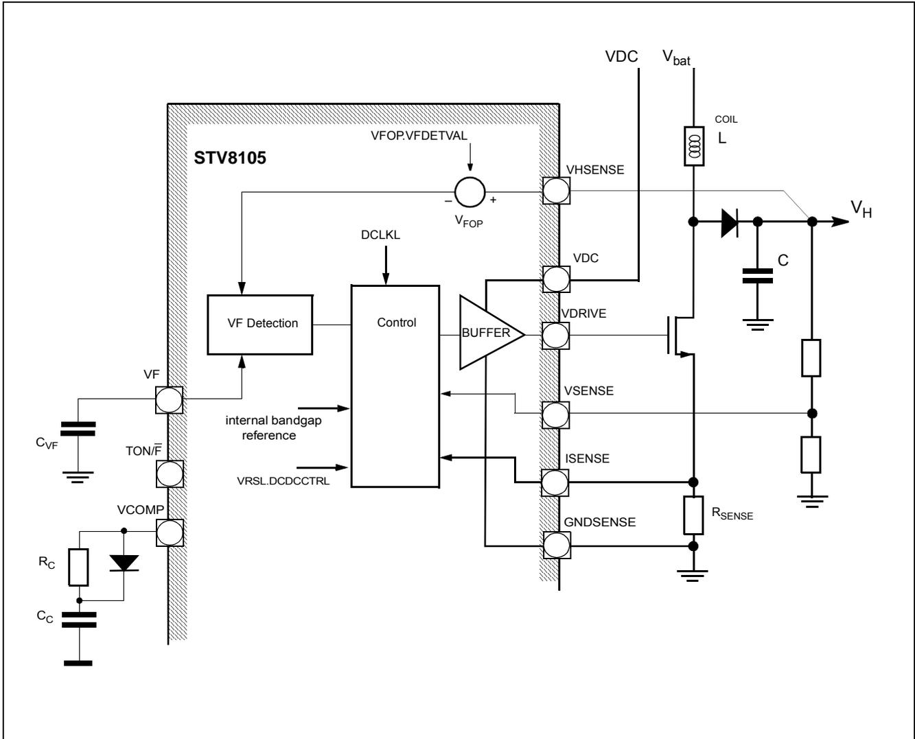
Output  $V_H$  is “clamped” to  $V_H$  Max. which equals a constant  $\times$  VBG at the time of VF detection. If  $V_H$  Max. is exceeded, then pad RCTRLB is pulled “High” to VDD by the STV8105 indicating a voltage fault.
