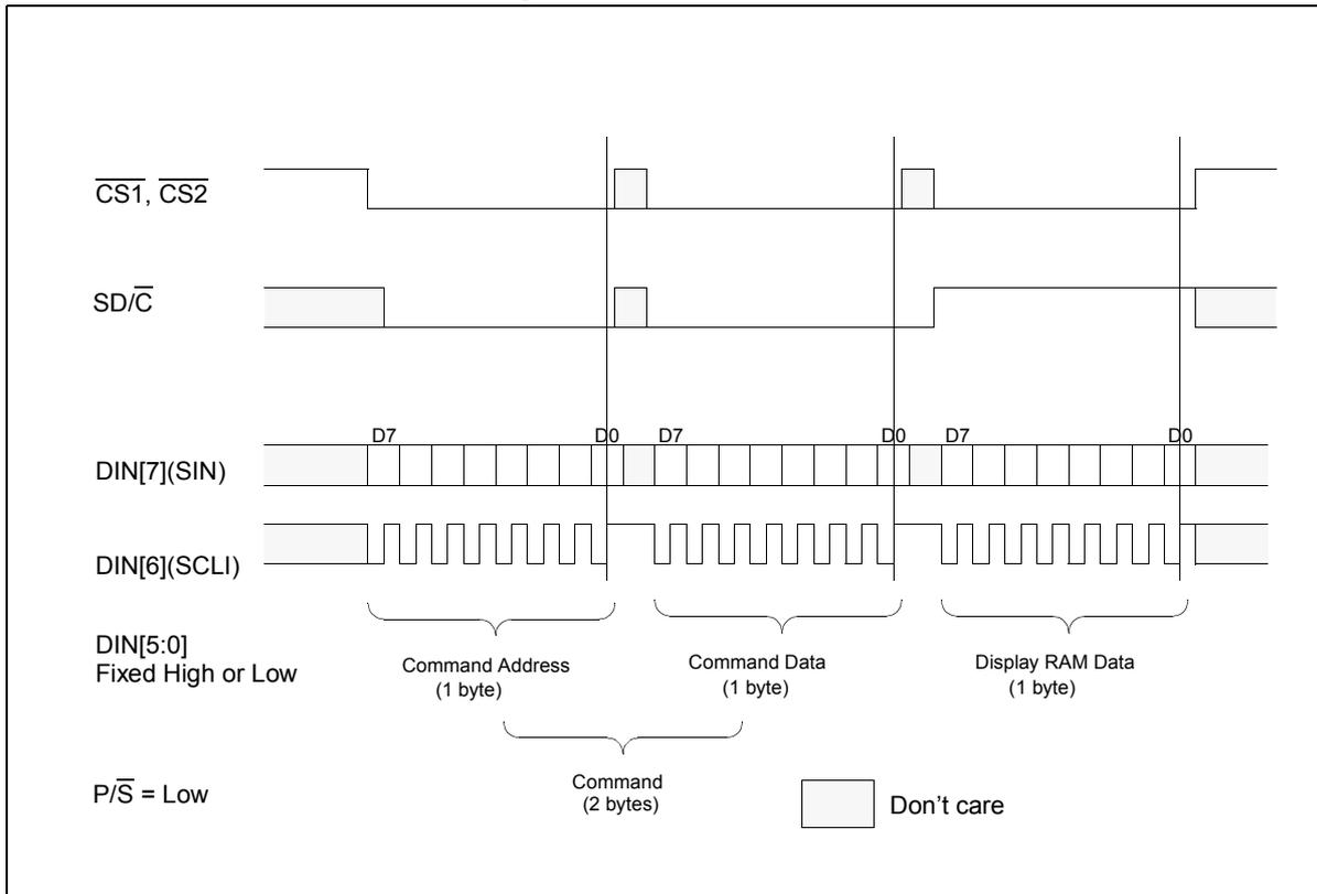
Figure 11: 4-wire Serial Interface Timing Diagram
