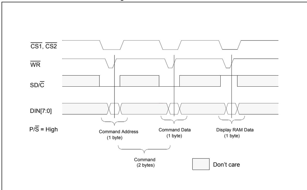
Figure 9: 8-bit Parallel Interface Timing Diagram
