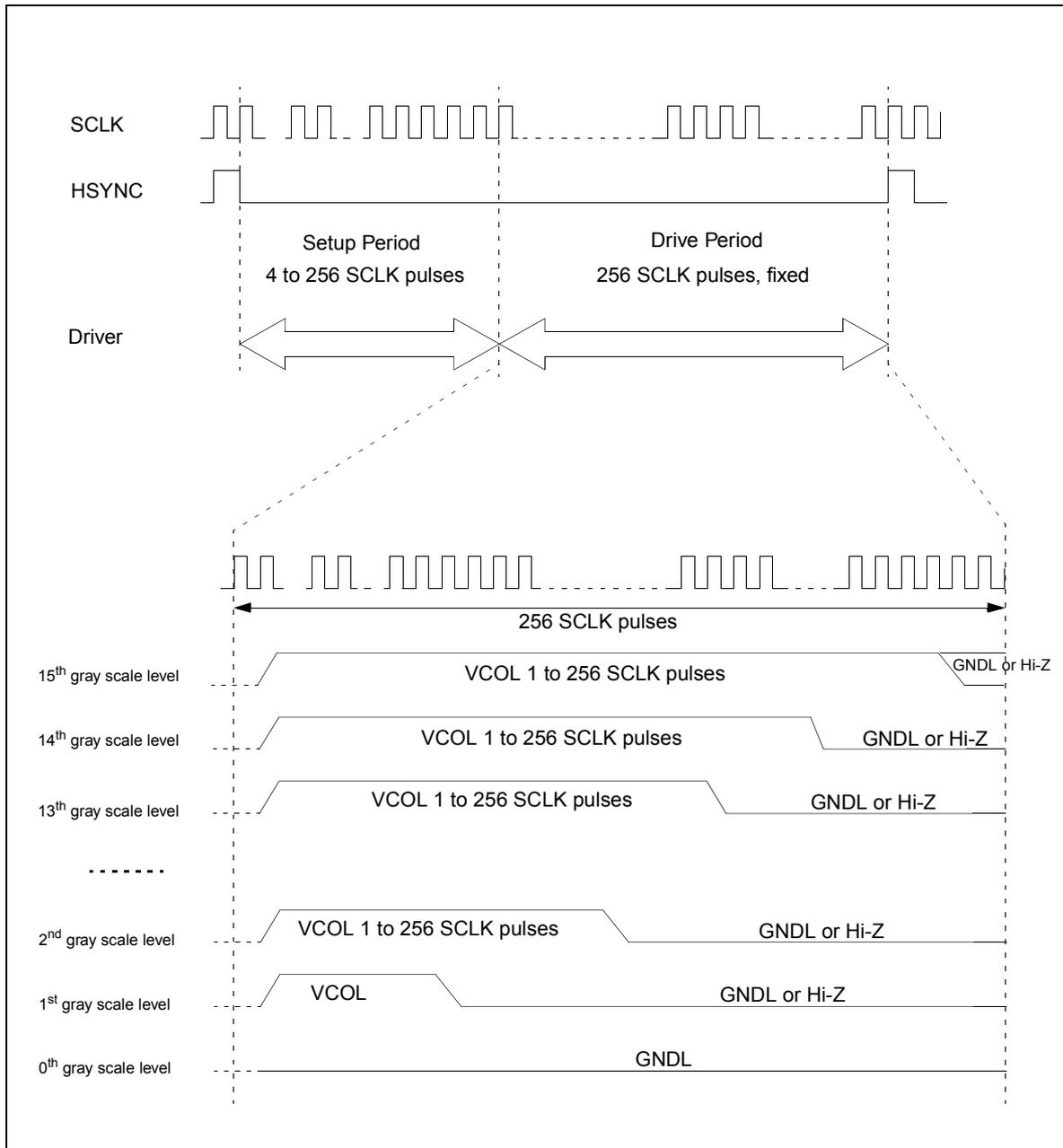
This mode uses the ODDx and EVENx, or ODDx only, lookup tables to define the column current sourcing time. There are 15 bytes corresponding to the 15 different, possible values of pixel data in Display RAM. When the pixel value is 0h, the column current source is off (to GNDL) for the entire drive period.
