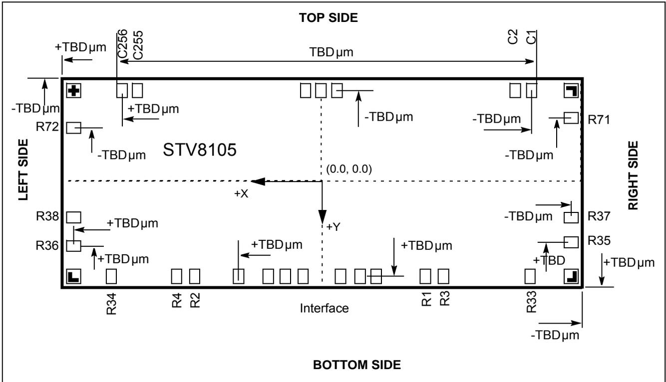
Figure 3: Alignment Mark Positions (Bump-side View)
