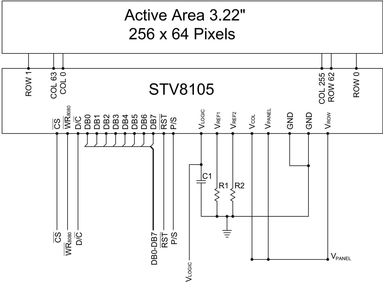
Figure 4. Connection Diagram
