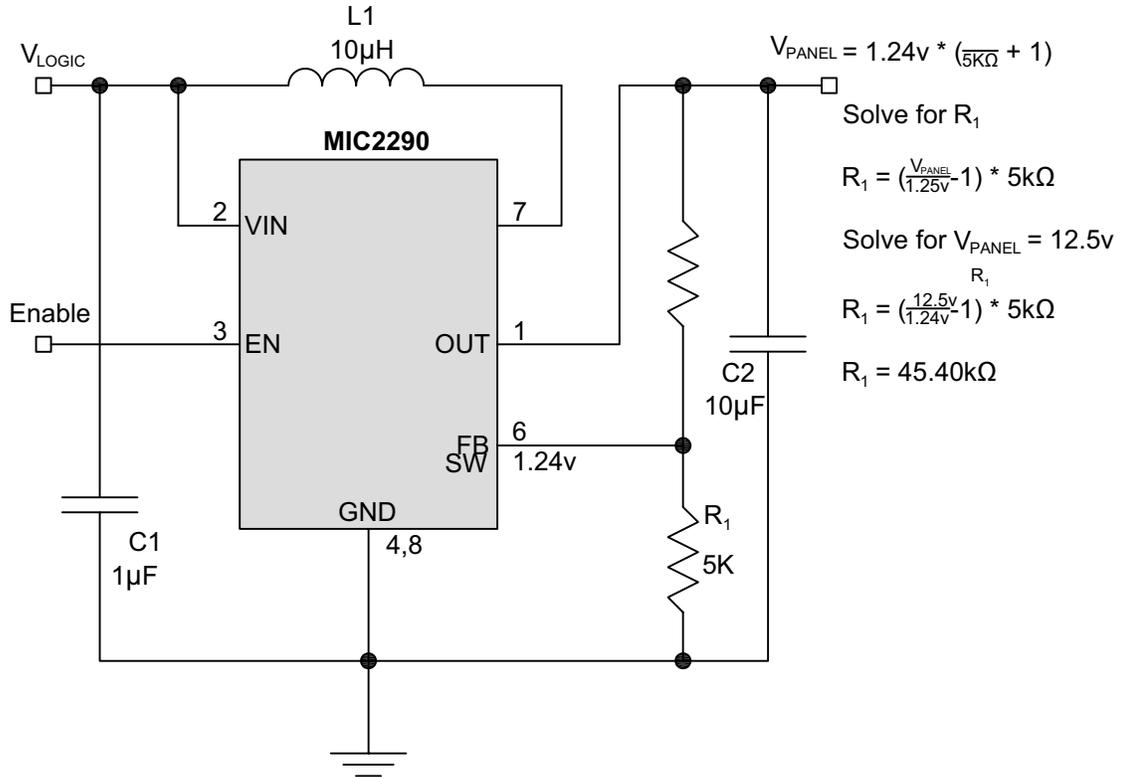
Figure 3. Circuit Example – External Supply for Display
