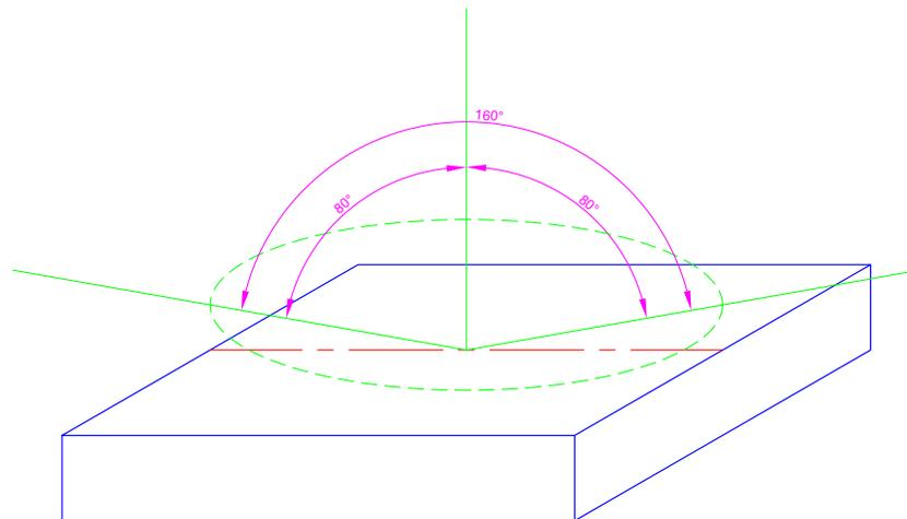
Figure 7. CFAL25664A-Y-B1 has a 160° Viewing Angle
