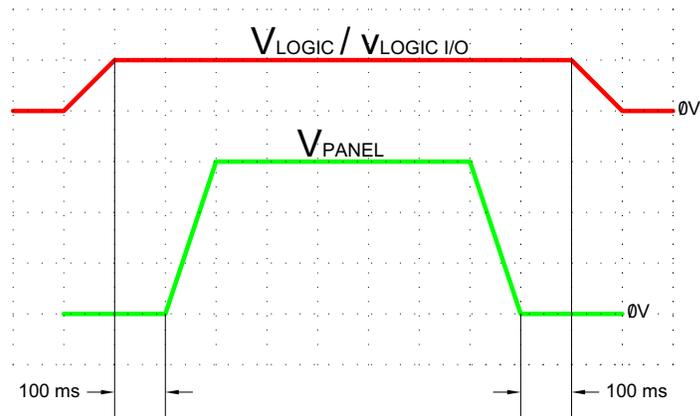
Figure 5. Power Up and Power Down Sequencing
