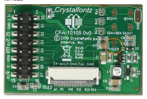
This jumper is shipped closed, tying V<sub>OLED</sub> high and thus enabled. To manually control V<sub>OLED</sub> Enable, open this jumper. Once open, Pin 11, VEN, on HOST will control V<sub>OLED</sub> Enable.
