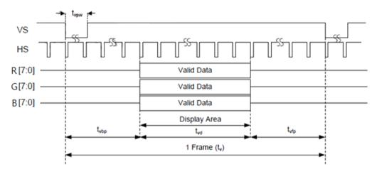
Figure 2 - 12.2. Parallel RGB in SYNC Mode (Vertical)
