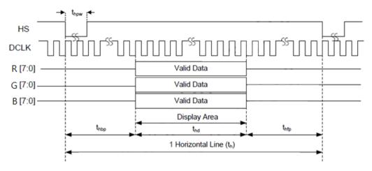
Figure 1 - Parallel RGB in SYNC Mode (Horizontal)
