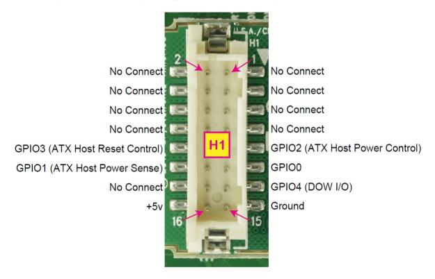
Figure 4. CFA-RS232 H1 Pin Assignments When Mounted to CFA Module
