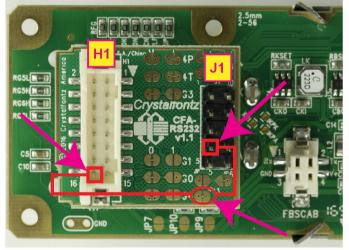
JP13 is closed by default, allowing the module to be powered by pin 4 on J1.
