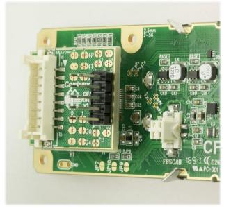
Figure 2. Angled View of CFA-RS232 Level Translator Mounted on CFA Module
