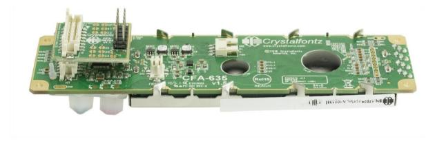
Figure 3. Side View of CFA-RS232 Level Translator Mounted on CFA Module
