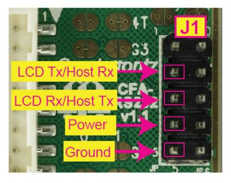
Figure 5. CFA-RS232 J1 Pin Assignments
