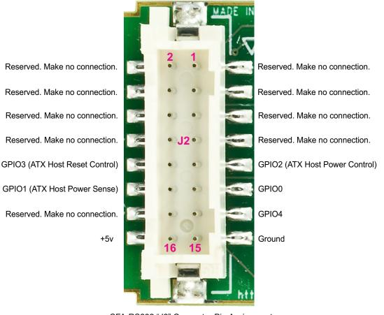
CFA-RS232 "J2" Connector Pin Assignments
