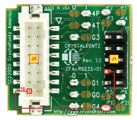
Jumper JP13 is closed by default at the factory. It allows power to be supplied to J1.
