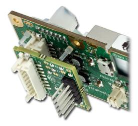
Photo Of CFA-RS232 Mounted On A Compatible Intelligent LCD Module (CFA735-\*\*\*-KT)
