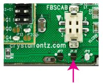
JP10 on Intelligent LCD Modules with simultaneous interfaces (CFA735 and CFA835 families) may be closed or open by factory default. If you are going to use USB interface while supplying power through "H1", you must open JP10 to prevent backpowering the USB.
