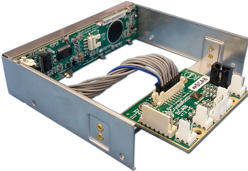
Figure 3. SCAB connected to a CrystalFontz CFA631 series LCD module using the WREXTY19 cable
