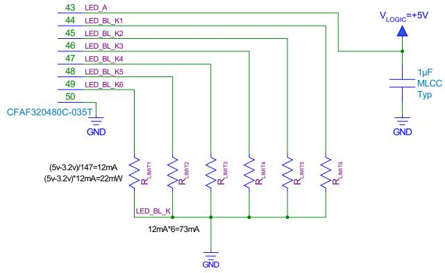
Figure 5. Typical LED Backlight Connections For "Always On"
