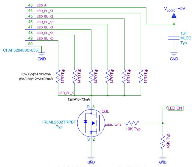
Figure 6. Typical LED Backlight Connections For PWM Dimming
