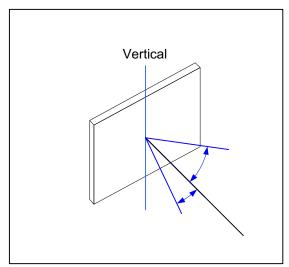
Figure 3. Definition Of Horizontal And Vertical Viewing Angles (CR>2)
