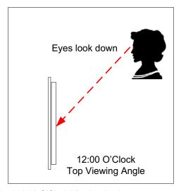
Figure 4. Definition Of 6:00 O'Clock And 12:00 O'Clock Viewing Angles
