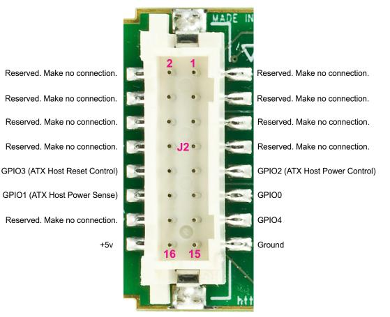
Figure 4. CFA-RS232 "J2" Connector Pin Assignments
