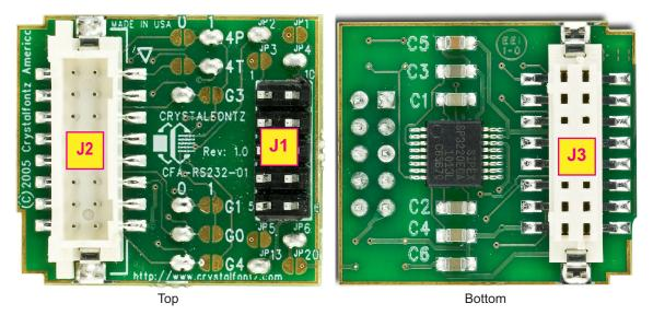
Figure 2. CFA-RS232 Top and Bottom View of Connectors
