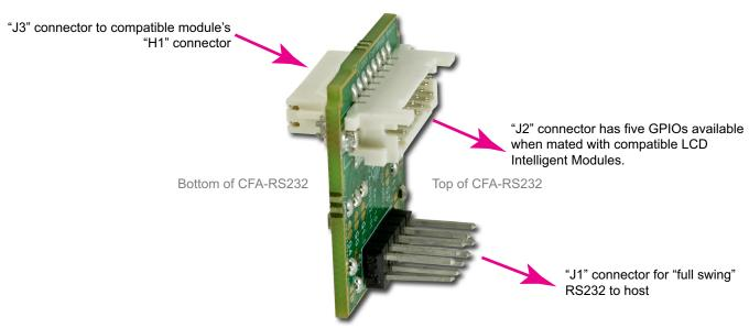
Figure 3. CFA-RS232 Side View of Connectors
