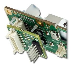
Figure 1. Photo Of CFA-RS232 Mounted On A Compatible Intelligent LCD Module (CFA735)
