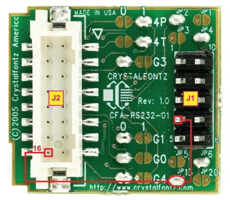
Jumper JP13 is closed by default at the factory. It allows power to be supplied to J1. J1 Default Pin Assignments – Pin 4 J1 Alternate Pin Assignments – Pin 7 J2 Pin Assignments – Pin 16
